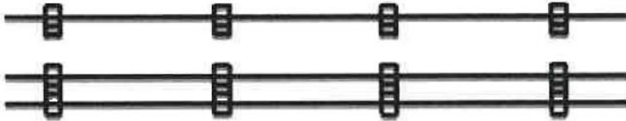
Figure 6 Special supporting structure with cable clamps attached to the ceiling or horizontally to a wall 4 or to steel profile and steel sheet. Design with F and DF clamps
